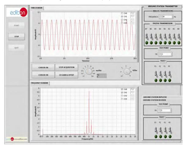
The screen below shows the use of the cursors to facilitate the analysis of the input signals. The screen shows the analysis of a 50 Hz signal.
