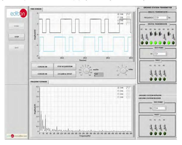
The screen below shows the analysis of a signal with an inserted fault in the Satellite Ground Transmitter Station. The faults can be configured at the right of the screen. In the image, the inserted fault is "FO"
