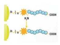
Functionally-activated microplates for covalent attachment of peptides, nucleic acids, and other biomolecules for ELISA and other plate-based assay techniques. These plates bind with functional groups such as amino (NH<sub>2</sub>), sulfhydryl (SH), carboxyl (COOH), and phosphate (PO<sub>4</sub>):
