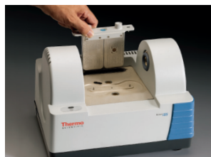
Easy desiccant replacement for maximum instrument protection
