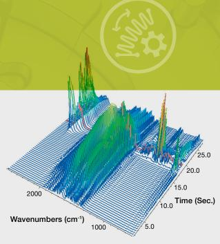
OMNIC Series software, unique Mercury TGA analysis package, and 3D displays allow you to quickly and efficiently extract useful information from TGA-IR (thermogravimetric infrared) and other time-based experiments
