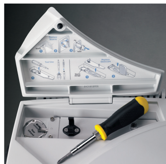
Optional tungsten halogen source and desiccant compartment are easily accessible
