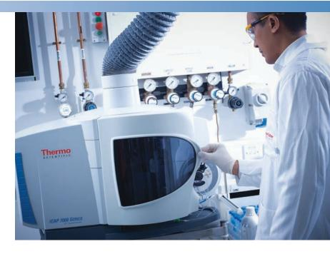
The Thermo Scientific™ iCAP™ 7600 ICP-OES is a powerful simultaneous spectrometer based on the core technologies of the Thermo Scientific iCAP 7000 Series ICP-OES to solve the challenges of the most demanding laboratory applications. The iCAP 7600 ICP-OES employs the latest technology developments to achieve exceptional performance and long term stability with capability for low gas consumption and high productivity to deliver the lowest cost analyses.
