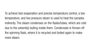
Steam temperature is controlled in two ways: 1) The pressure in the outer chamber (at point A) is set to boil water at the desired temperature, while 2) The temperature of the outer chamber is precisely controlled at or below the set temperature.
