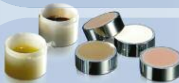
Collection pot for safe loading of pressed powders and liquids
