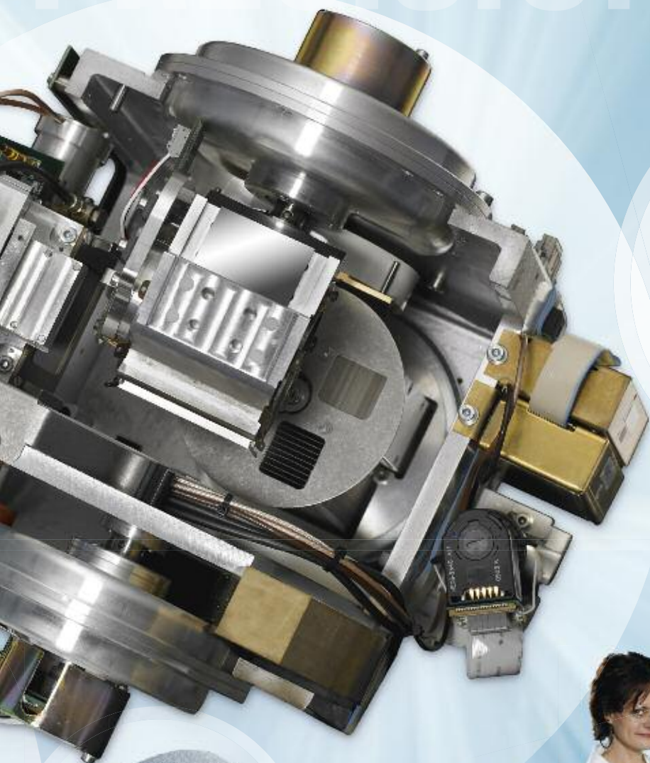
6th generation universal gearless goniometer
